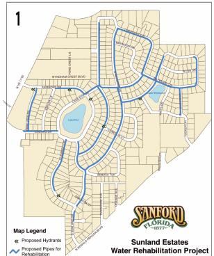
be increased from 4" to 6" and new fire hydrants are to be installed to improve fire protection. The water line replacement using pipe bursting in Sunland started in August. Two additional subdivisions will be replaced using the technology.
